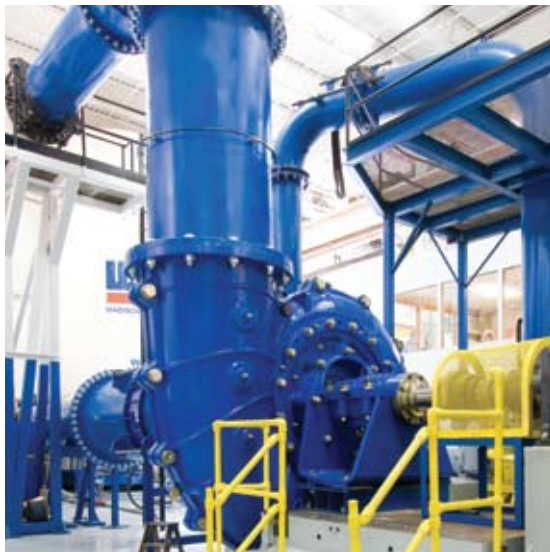
Far right: A Warman 600 HTP being prepared for hydraulic testing. The massive rib reinforced casing and 102,000 lb bare weight illustrate the robust design and inherent safety of this 580 psi rated pump
