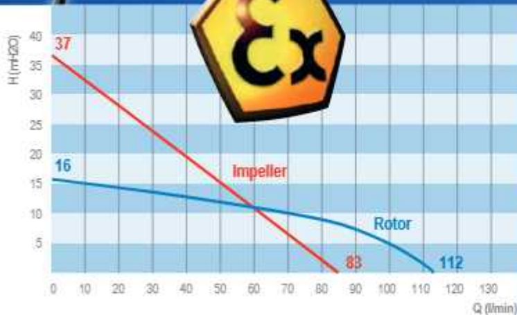
JP-480, 230 V AC, JP-SS 41-1000, test media water 20 °C, pressure pipe 1", oval gear meter, measured values ± 5%
